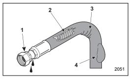
Figure 3-3 Hydraulic Hose Damage
